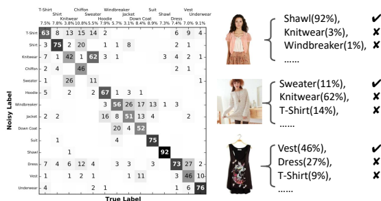
Fig. 2: The transition matrix of Clothing1M copied from [38]. The distribution of noisy labels are highly imbalanced. Some classes are almost clean (e.g. Shawl) while some classes has more mislabeled samples than correct labels (e.g. Sweater).
