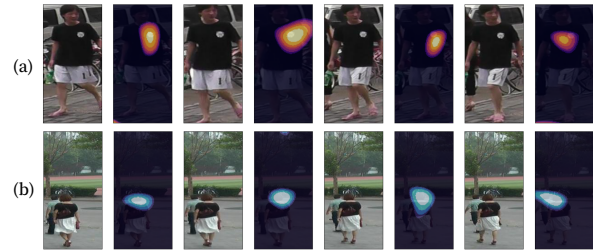
Fig. 11: Visualization of attribute-aware proxies for two different pedestrians on MARS. Attention heat maps of four consecutive frames from the AAP embedding module on Stage I are displayed.
