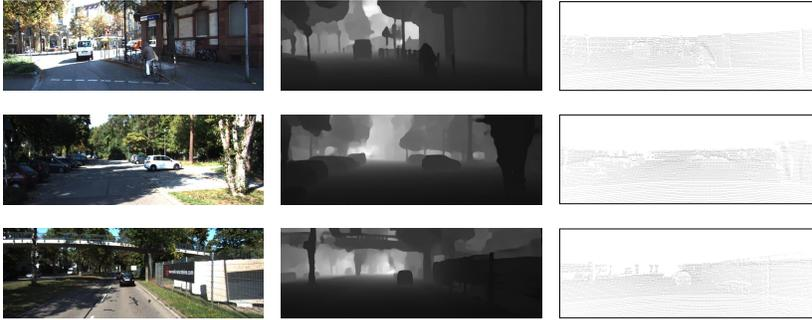
**Fig. 2.** Examples of the enhanced dense depth maps generated by a stereo matching model [22]. We use these depth maps as complementary data to the sparse ground truth depth maps. The left column contains RGB images, while the middle and right column show the enhanced depth maps and sparse ground truth, respectively.
