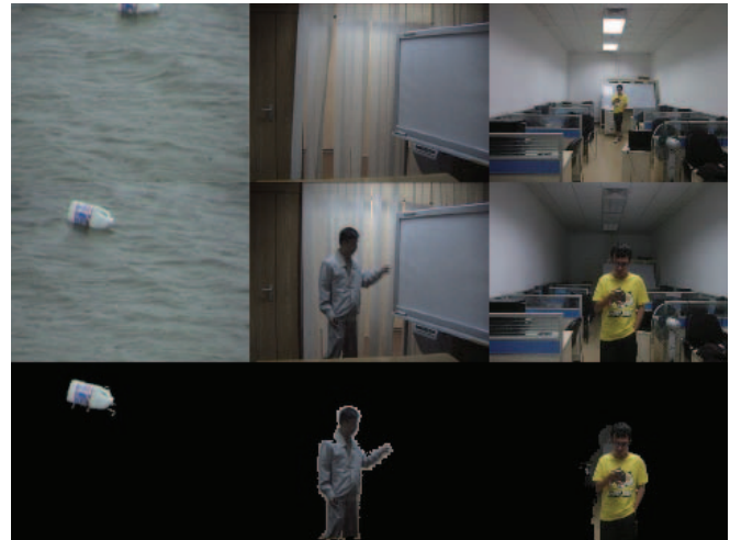
Fig. 1. Some challenging scenarios for foreground object extraction are handled by our approach: (i) a floating bottle with randomly dynamic water (in the left column), (ii) waving curtains around a person (in the middle column), and (iii) sudden light changing (in the right column).
