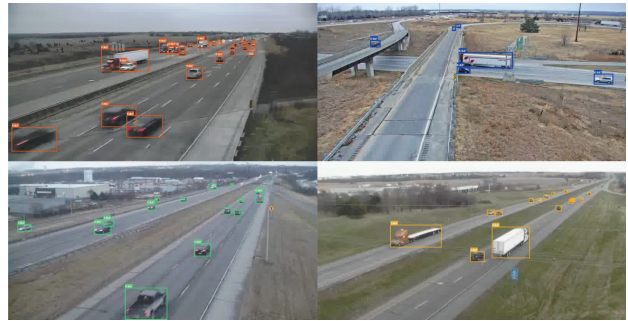
Figure 3. Examples of detection results, which from video 13, 18, 23 and 28 in track4 test dataset. From the visualization, we observe that small targets can be predicted accurately.
