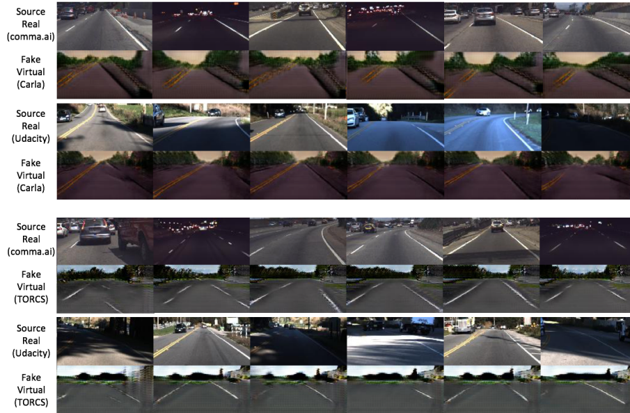
Fig. 7. Image generation results of DU-Drive. Information not critical to driving behavior, e.g. day/night lighting condition and the view beyond road boundary, is unified. Driving critical cues like lane markings are well preserved.
